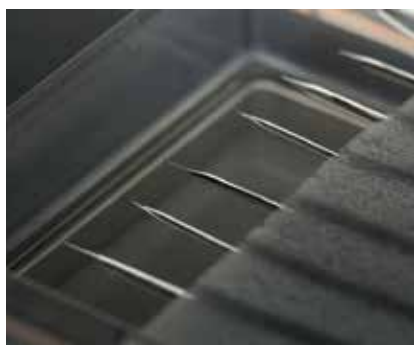
Conductive diamond in the form of needle-like microelectrodes makes excellent biocompatible sensors. © 2018 Yasuaki Einaga
