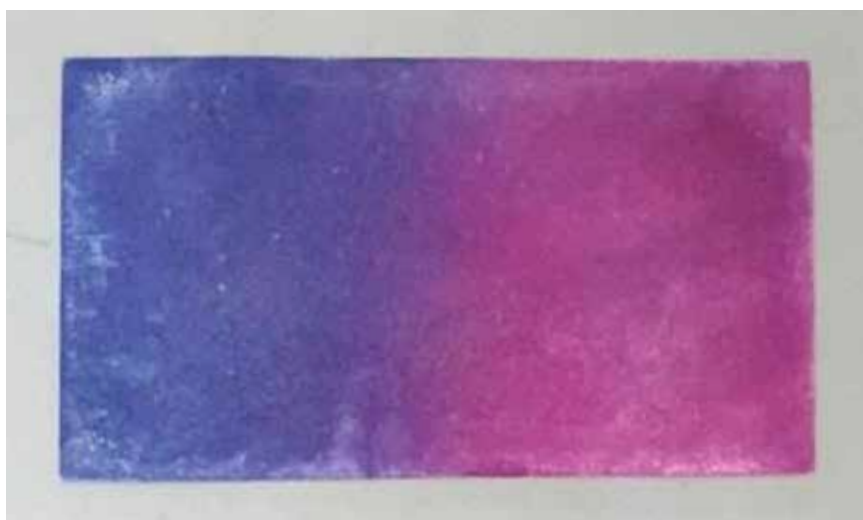
The polydiacetylene material developed by Yuya Oaki and his team changes color based on responses to external stimuli such as temperature.
